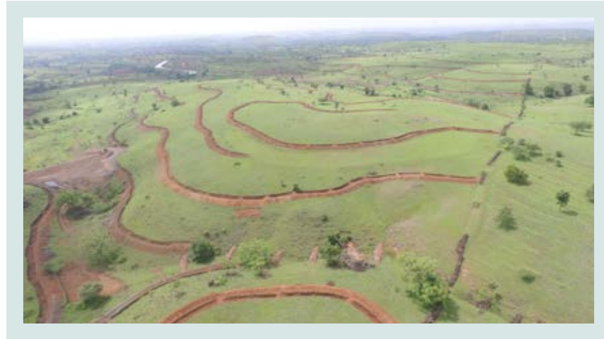
Water absorption trenches and percolation tank for ground water recharge, Narayangavhan village, Parner block, Ahmednagar district
