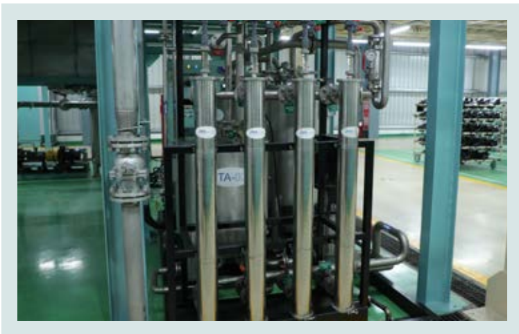
Advanced effluent recycling method deployed – electro deposition reverse osmosis
